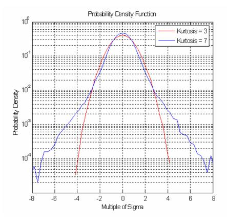
Using traditional (ISTA/ ASTM) random vibration to include these peaks, one would have to increase the power of the test,  $G_{RMS}$ , across the entire frequency spectrum. This clearly constitutes an over-test condition. The need for the higher velocities that are needed to test to higher Kurtosis adds design implications and higher cost to vibration test system
