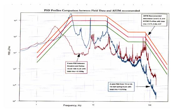
Because the PSD is a statistical average intensity, we suspected that the actual road peak accelerations would differ greatly from the average, specifically in those frequency bands where the average is high and represents typical fundamental frequency of truck transport.
