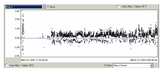
From the above scatter plot covering the entire transport exposure, the initial hour contained peak events, some exceeding 1.5 Gs and number reaching 2 to 3 Gs. This represents severe road sections of speed bumps, potholes, railroad tracks or curbs. Loading and handling shocks could contribute It should not be ignored in the test protocols for the packaged product. Truck suspension and driver behavior are also variables to be investigated.
