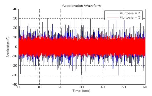
The ISTA/ASTM random vibration test spectra are all based on 3 sigma-limited Gaussian distribution (red curve) for which coincidentally, is Kurtosis=3. The PSD, however, and the root of its area,  $G_{RMS}$ , do not indicate in any way, the severity of peak accelerations that differ from the standard Gaussian normal distribution used for test specifications. The Gaussian PPDF (peak probability distribution function) is shown in RED in the following figure.
