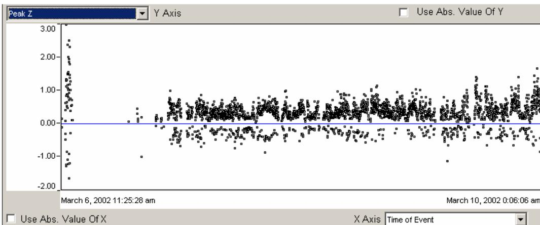
From the above scatter plot covering the entire transport exposure, the initial hour contained peak events, some exceeding 1.5 Gs and number reaching 2 to 3 Gs. This represents severe road sections of speed bumps, potholes, railroad tracks or curbs. Loading and handling shocks could contribute. It should not be ignored in the test protocols for the packaged product. Truck suspension and driver behavior are also variables to be investigated.
