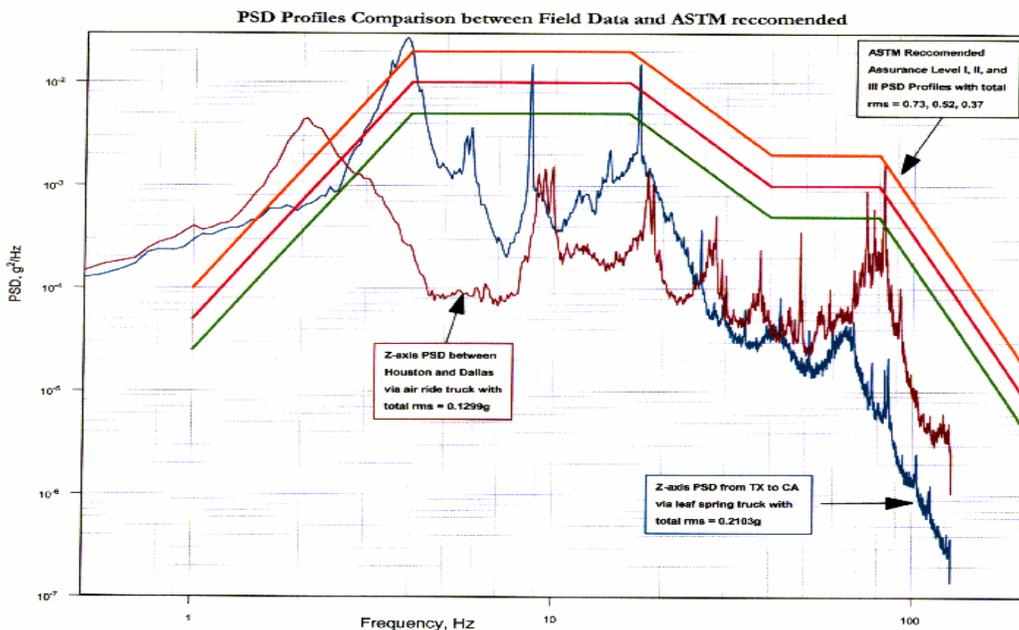
Because the PSD is a statistical average intensity, we suspected that the actual road peak accelerations would differ greatly from the average, specifically in those frequency bands where the average is high and represents typical fundamental frequency of truck transport.
