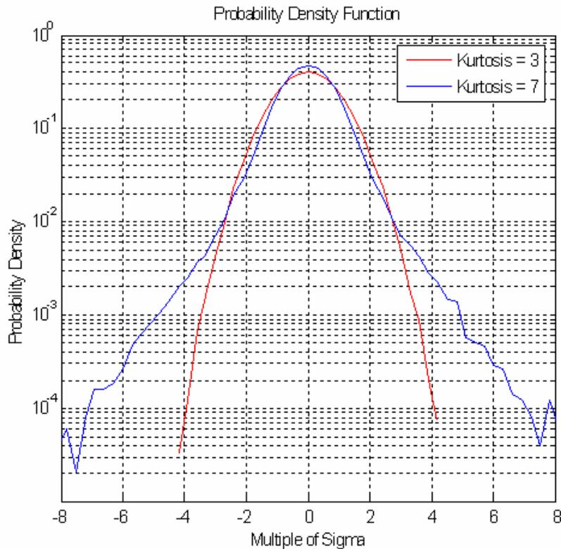
Using traditional (ISTA/ ASTM) random vibration to include these peaks, one would have to increase the power of the test,  $G_{RMS}$ , across the entire frequency spectrum. This clearly constitutes an over-test condition. The need for the higher velocities that are needed to test to higher Kurtosis adds design implications and higher cost to vibration test system
