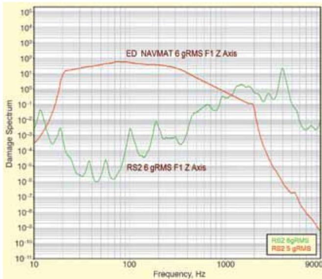
Figure xx shows two response FDS plots from different fixtures on an RS machine. Table shows different FDS transmissibilities at different gRMS setpoints. Shaker control time histories could also generate FDS plots and  $\Sigma_{FDS}$  characterizing the shaker excitation or an EUE. With a test profile generated from the EUE, refinements to m and Q produce FDS and  $\Sigma_{FDS}$
