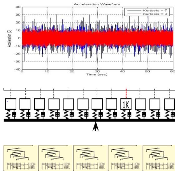
The rainflow cycle counted damage at each RIRDF (Smallwood) is represented below in the distributions at each SDoF.
