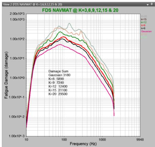
The companion tool to the FDS is Vibration Research's patented Kurtosion<sup>®</sup>, which captures the damage from all excitations, non-Gaussian and non-stationary excitations, in contrast to these short-comings of traditional FFT-based PSD and gRMS tools.
